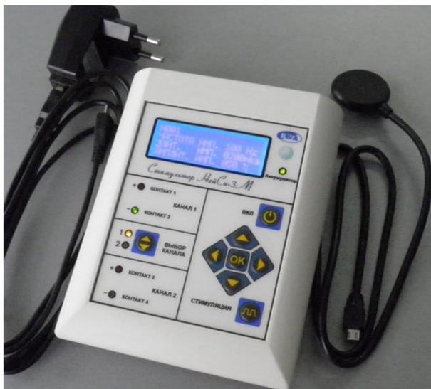
Figure 4. External control panel with a telemetry antenna.
